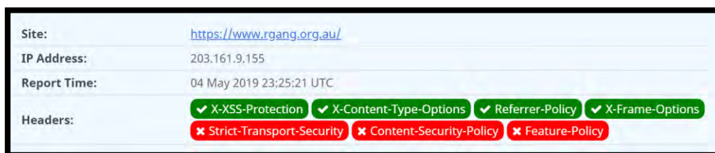
Screenshot 9. Headers missing on www.rgang.org.au
